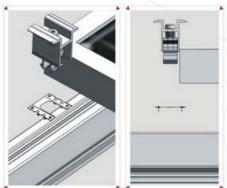
Slide grounding clip intomodules clamp slot of rail. Torque modules in place on top of clip. Nibs will penetrate rail anodization and create grounding path through rail.
