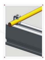
Place the Lug portion in the slot of rail, Fix the lug to the rail using three 6 x 20 mm tapping screws. The tapping screws make a gastight mechanical connection and ensure good electrical connection between the aluminum rail and the lug through the stainless steel tapping screws
