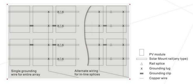
Place grounding clips, Lugs, and copper wire (6 –10 AWG) as shown. Place a loop in the wire around splices to prevent tension. Be sure wiring between rails is not taut.
